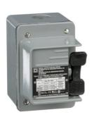
Switch, manual, 30A, 3 pole, 10 HP at 575 VAC, three phase, toggle operated, no indicator, NEMA 4, two conduit opening
